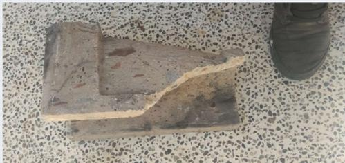
Why scary? Because it's a solid chunk of cement that fell off the building. Two have fallen - one last year and one this year. Irving replaced them with PVC which can be inserted further into the building drain holes and hence stand a better chance of not falling to begin with. And if one were to fall out, it wouldn't hurt someone.
