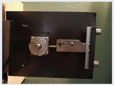
We realize that none of the things we have done thus far mean anything because the safe design is such that the back most dial plate is larger than all the others - so we only hear things that help us to detect the last of the three digits in the combination. Which helps not a whit because if you know the first two, you can just slowly turn the knob and find the last number in the combo anyway.
